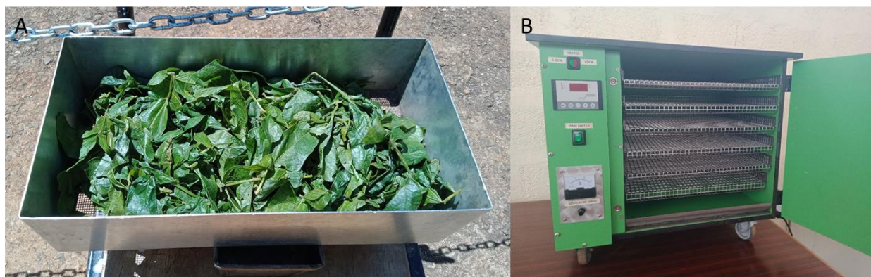
Figure 4: Other techniques of dehydration of cowpea leaves. A-Sun-drying of blanched cowpea leaves, B- Forced air ventilation oven drier
