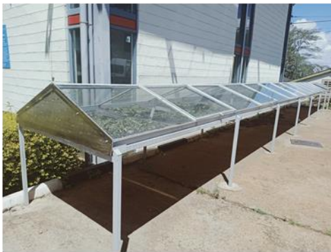
Tunnel solar drier
